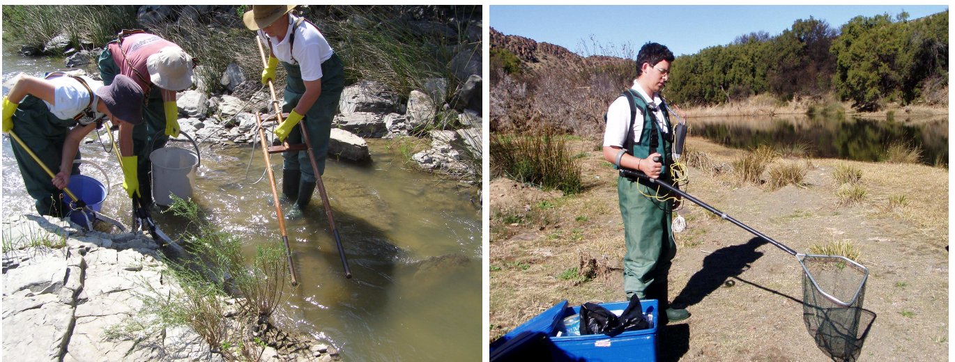
Figure 4.2: The “old” parallel fork electroshocker powered by a 220 V AC, 2 kva Yamaha generator (left) and the “new” Samus 725G backpack-electroshocker used from August 2006 onwards (right).
